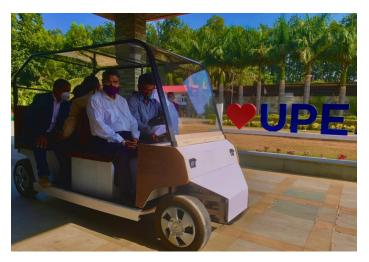
The electric vehicle, U-BAHN, has been developed in nine days on the campus with a cost of Rs.2 lakh. It can travel at a speed of 25 kms per hour and will be embedded with an IoT-based system to help the driver know about the pickup and drop location
